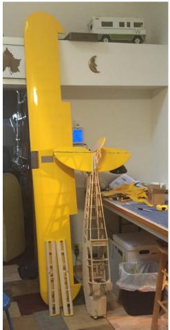
The radio controls are removed for now. The ailerons are sitting in front of the wing. Those will be covered next. Then I will work of the fuselage and fin after that. There are a few parts I have to paint. The covering does not
